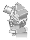
7. Move the air cleaner housing cover and remove the cover from the air cleaner housing.
